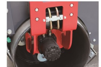
Hydraulic motor direct drive, double drum driving
