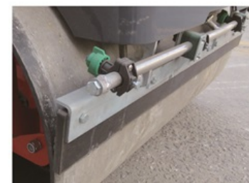
Double drum water spraying, scraper cleaning
