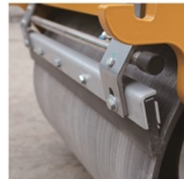
Double drum water spraying scraper cleaning
