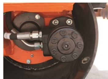
Hydraulic motor, double drum driving
