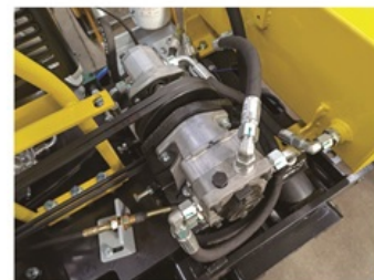
Imported hydraulic pump, infinitely variable speed
