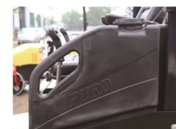
Extra-large plastic water tank, free from corrosion and easy to spray water
