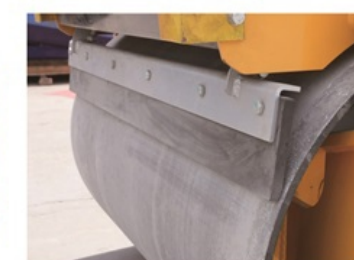
Double drum water spraying scraper cleaning
