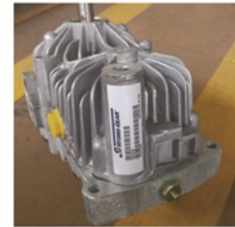
Imported hydrostatic pump infinitely variable speed
