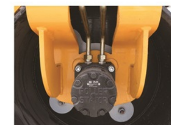
Hydraulic motor, double drum driving
