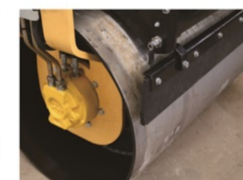
Wear-resistant scraper, can lift up
