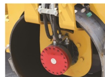
Imported plunger motors, double drums hydraulic driving
