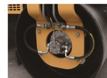
Hydraulic vibration is driven by imported motor
