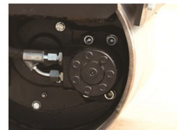
Hydraulic motor, double drum driving
