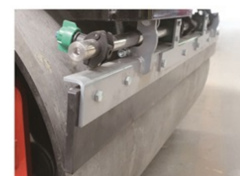
Double drum water spraying, scraper cleaning
