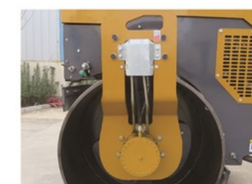
Double drums hydraulic motors driving
