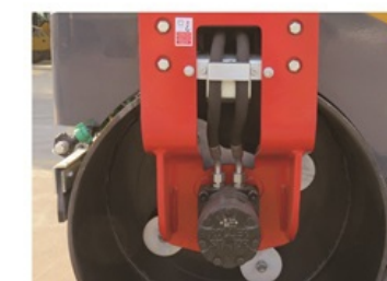
Imported danfoss hydraulic motor direct drive
