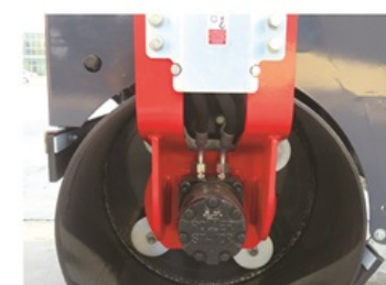
Hydraulic vibration is driven by imported motor
