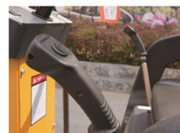
Double control handles with vibration button
