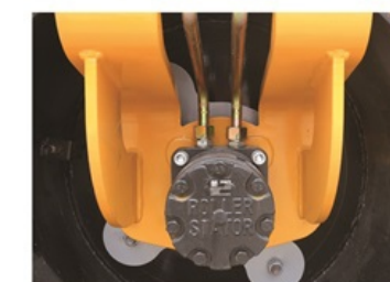
Hydraulic motor, double drum driving
