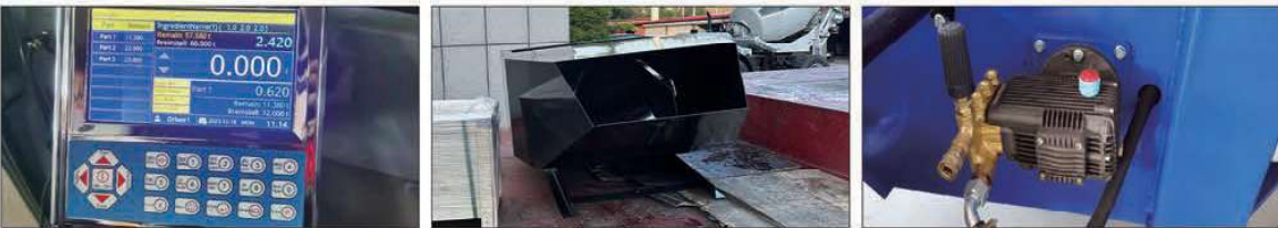
Electronic hydraulic weighing system Cement hopper Hydraulic car washing machines
